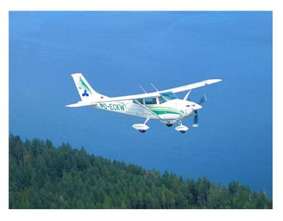
Regardless of the nearly 1,500 nm journey or the 75 minutes of holding added to the flight time, the performance and fuel efficiency of the SMA engine was remarkable. Airborne for a total of nine hours twenty five minutes (9:25) the SMA compression-ignition powered Skylane consumed a total of 80 gallons Jet-A fuel; giving the crew approximately 18 miles per gallon fuel burn (ignoring an hour of hold time).
