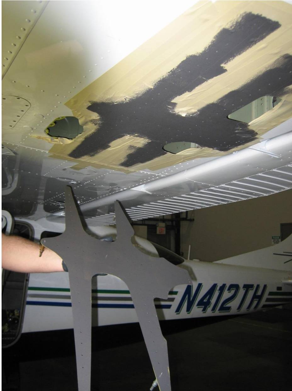
Figure 8: Sealant Coated Faying Surfaces
