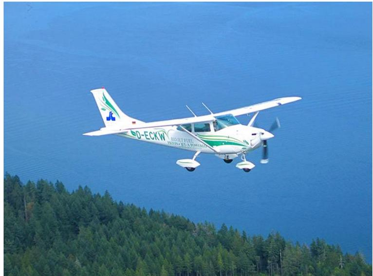
Regardless of the nearly 1,500 nm journey or the 75 minutes of holding added to the flight time, the performance and fuel efficiency of the SMA engine was remarkable. Airborne for a total of nine hours twenty five minutes (9:25) the SMA compression-ignition powered Skylane consumed a total of 80 gallons Jet-A fuel; giving the crew approximately 18 miles per gallon fuel burn (ignoring an hour of hold time).
