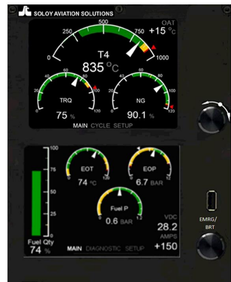
The Electronic Engine Management System contains two separate displays – the upper Primary Display (LCD #1) and the lower Secondary Display (LCD #2).
