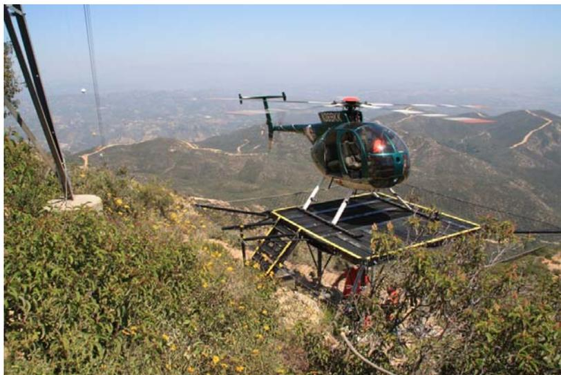
SDGE personnel found that assembly of the Heliports is quick with the patented telescoping legs that adjust to any terrain and lock into position. Made of heat-treated aluminum alloys with stainless steel cables and pins, the Heliport is designed to transfer the load from the landing helicopter throughout the structure, minimizing the loading on any one structural member. The Heliport has a stable sling load and can be set in place with low environmental impact and no site preparation.
