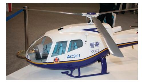
forest firefighting and other general aviation services. The helicopter fuselage and rotor blades are built of composite materials. The AC311 comes equipped with an advanced avionics system and the cabin has sound absorption materials.
